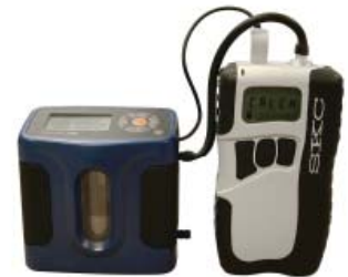
Multiple-point calibration train with CalChek; do not place sample medium in line.
