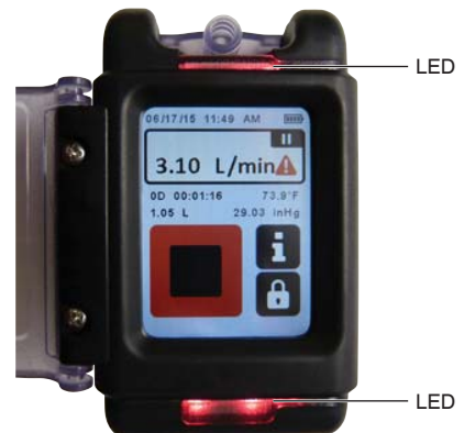
Figure 6. Red, flashing = Flow fault
