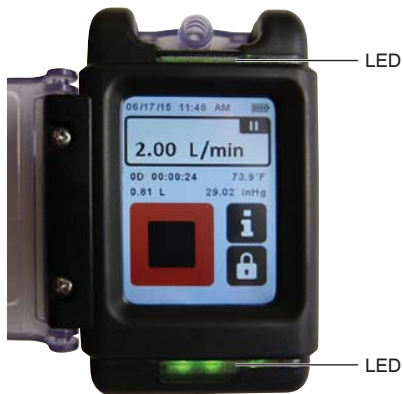
Figure 5. Green, flashing = Pump or schedule running
